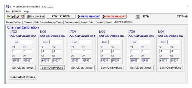
This tab shows the current calibration/scaling parameters for the input.
