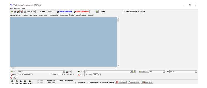
In the terminal window you can see the output from the unit and type commands to the unit.
