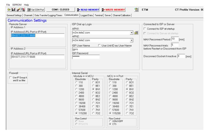
This section has settings which controls how the wireless modem communicates over the internet with a server. There are also settings for the communication with the internal module.
