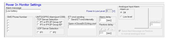
The unit can send an alarm when the unit's supply voltage level has fallen below a specific level. This can be used as a warning for backup battery, solar or mains power failure applications.
